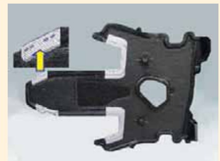
Joining of plastic parts with aluminium sheets on the bottom of the vehicle (replaces rivets/screws)
