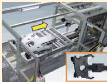
Joining of plastic parts with aluminium sheets on the bottom of the vehicle (replaces rivets/screws)
