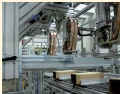
Stapling of PAL-box sleeves
