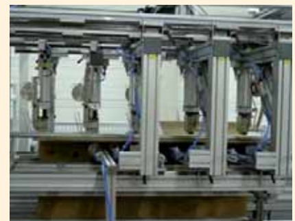
Stapling of sleeves to ready-made PAL-box
