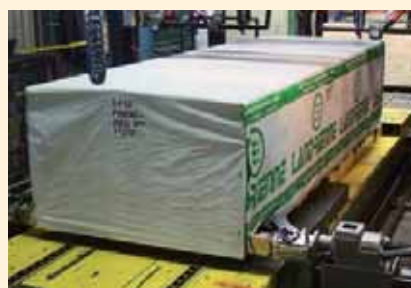
Fully automatic attachment of a protective tarp onto pre-cut wood
